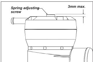
spring pre-load adjustment is not critical and is it possible to use the Mach 2 valves straight out of the box without adjustment. However, you can use the adjustment to fine-tune throttle response. Generally speaking, the hardest spring pre-load you can run without causing compressor surge (fluttering sound when lifting off the throttle) is ideal.
