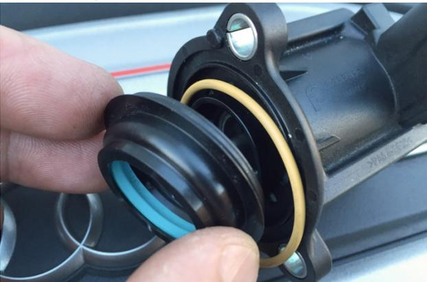
Store the piston, shroud and spring as these are not used in the DVX, and keep the yellow o-ring and screws for the DVX installation.
