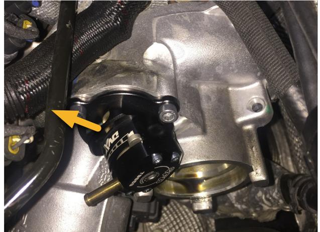
Push the supplied vacuum hose onto the barb on the remote solenoid mounting block, then install the mounting block onto the engine's vacuum pump as shown below. There is an un-used threaded hole where the supplied M6 x 25 screw fits (white arrow), and a blank hole where the silver dowel on the mounting block locates (red arrow).
