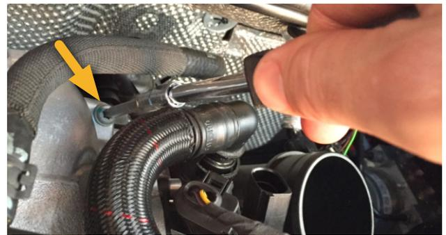
Rotate the top of the intake elbow towards the firewall to disengage it from the turbo as shown below.
