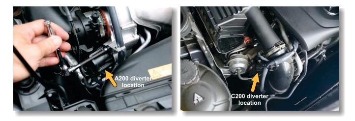
• Using a 5mm hex driver/key, undo the 3 screws holding the diverter - take care not to drop them!
