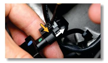
• Separate the factory valve mechanism from the solenoid body by pulling on the plastic sleeve ( >) that surrounds the diaphragm - don't pull on the valve itself as the diaphragm may tear.
