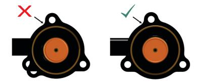
• Install the VTA assembly onto the turbo using the supplied longer screws. Because of the asymmetric bolt holes, the assembly can only be installed in one orientation.
